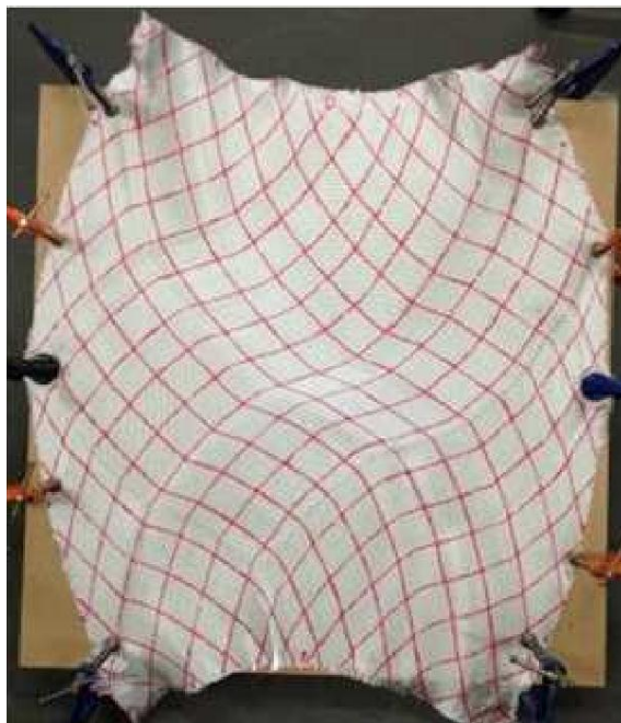
Figure 1. Sheared woven roving glass engineering fabric circumferentially [19].
