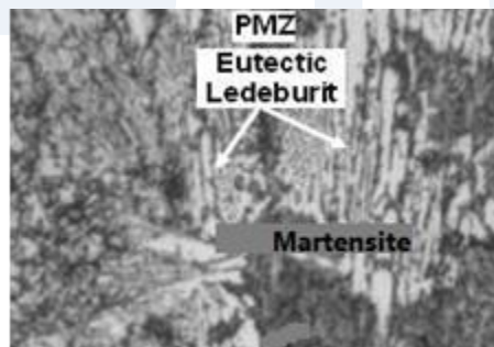
Figure (4) partial melting zone (Pouranvari, 2008)
